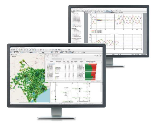
PowerFactory is also perfectly suited to transmission system operation planning. It integrates a comprehensive set of tools to support automatic and parallel grid security analysis such as ENTSO-E D2CF/DACF/IDCF, and outage planning. Multiple interfaces (API, DGS, CIM) and flexible scripting languages (DPL, Python) enable smooth integration with existing systems, and compliance with the ENTSO-E CGMES data exchange standard.
