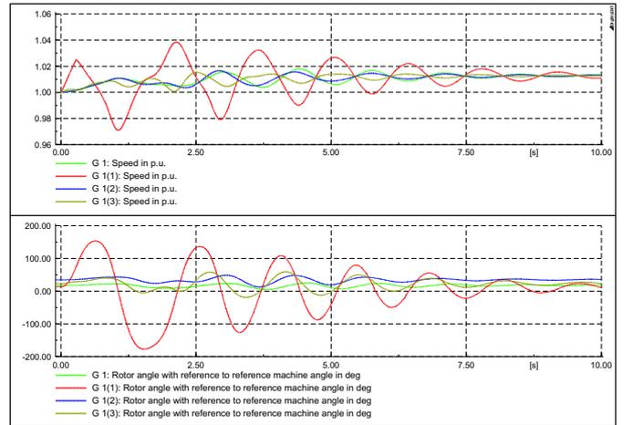
Fig. 7: Stability limit in the base case; Rotor angle and speed of generators in all four areas.
