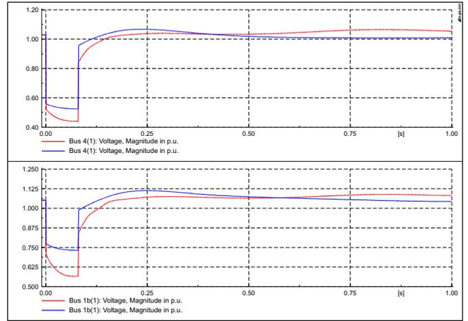
Fig. 11: Voltage Recovery of the system to a fault of 80 ms for Case 1 and Case 2 by comparison.
