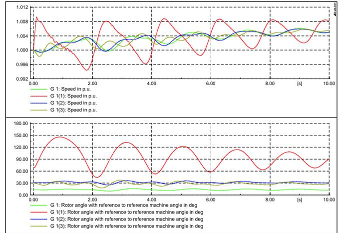
Fig. 14: Stability limit in the Case 4 at  $t_{CCT} = 101$  ms; Rotor angle and speed of generators in all four areas.
