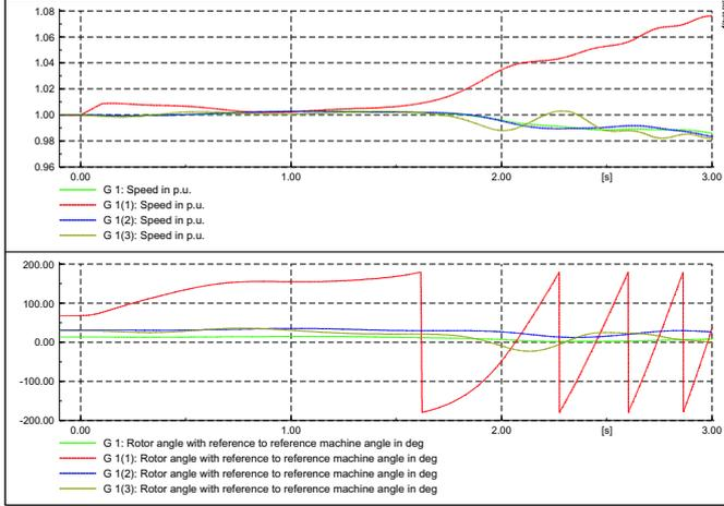
Fig. 8: Case 1 after a fault of  $t = 100 \text{ ms} > t_{CCT}$ ; Rotor angle and speed of generators in all four areas.
