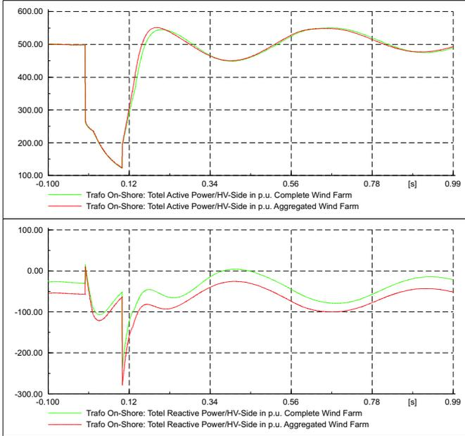
Fig. 4: Comparison of the complete wind farm to the aggregated wind farm
