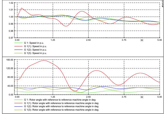
Fig. 9: Stability limit in the Case 2 at  $t_{CCT} = 146 \text{ ms}$ ; Rotor angle and speed of generators in all four areas.
