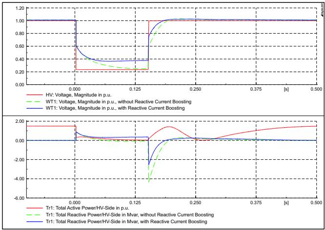
Fig. 2: Voltages, Active and Reactive Power at the PCC during a 3-phase fault with (solid) and without (dashed) reactive current boosting.
