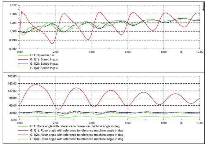
Fig. 14: Stability limit in the Case 4 at  $t_{CCT} = 101$  ms; Rotor angle and speed of generators in all four areas.
