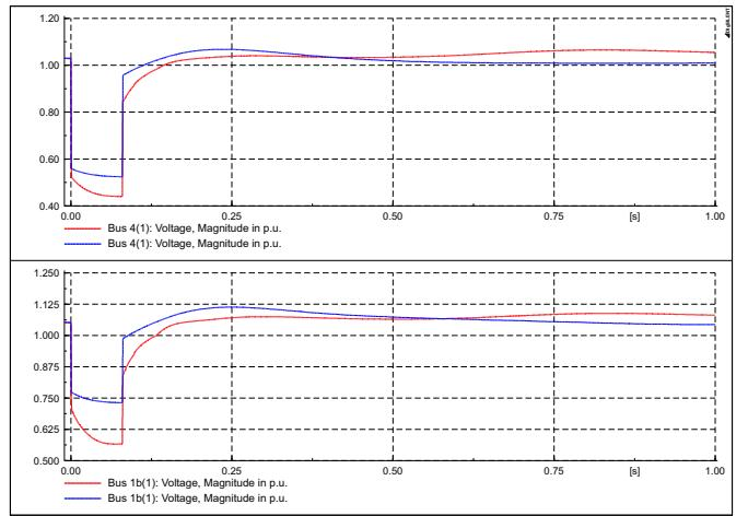
Fig. 11: Voltage Recovery of the system to a fault of 80 ms for Case 1 and Case 2 by comparison.
