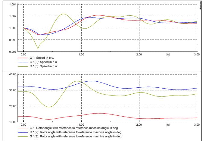
Fig. 12: Speed Response of the system to a fault of 250 ms for Case 3.
