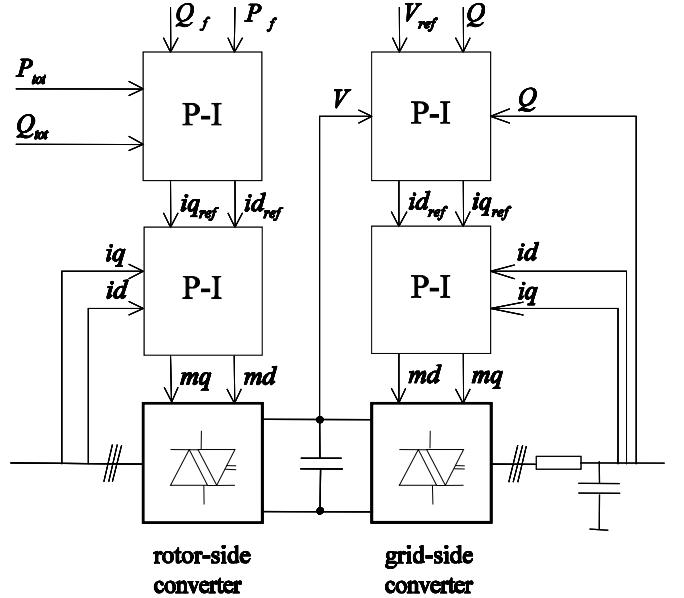
Fig. 3: Electrical Control Concept of the DFIG
