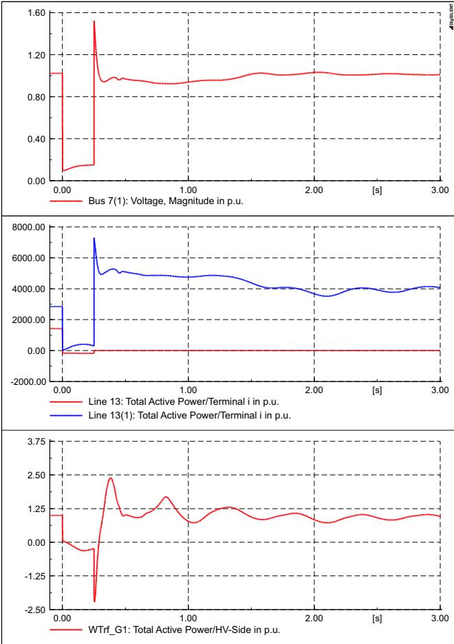
Fig. 13: DFIG Response to a fault of 250 ms with active voltage control.
